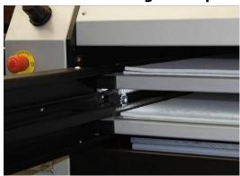
Unscrew and remove the screw TFM5-12 + Washer.
