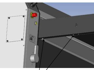
Screw and tighten the 4 screws M8-12 curved
