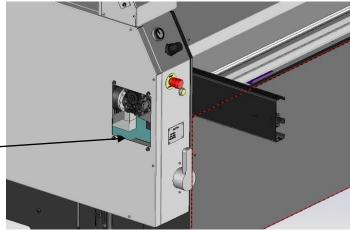
Handing over the hatch for the arm support cables within the enclosure
