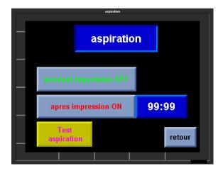
Allows the aspiration motor test and adjust its operation during the cycle
