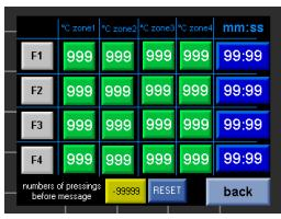
Set the customer pre-sets parameters and also the numbers of pressings before the message « change felts »
