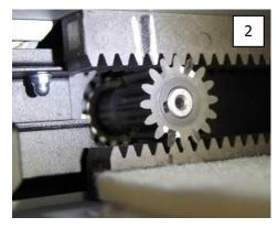
Remove the motor pinion pulling. If necessary, relieve the weight of the upper frame by slightly raising.
