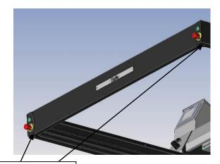
Screw and tighten the 4 screws curved M5-12
