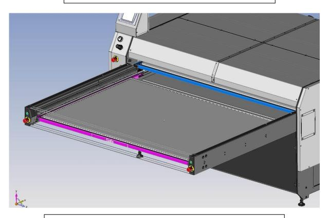
Reassemble the motor pinion ensuring continuity pins made on both the pinion and the rack. If necessary, relieve the weight of the upper frame by lifting slightly.
