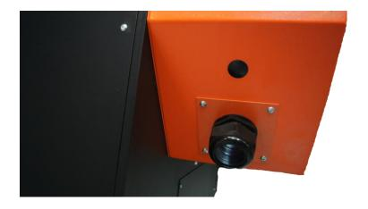
Pass the cable into the electrical cabinet and connect the 3 phases and the earth
