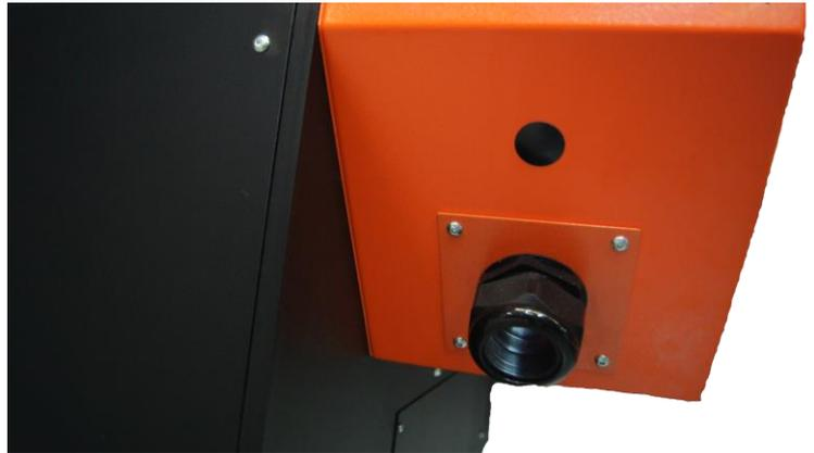
Pass the cable into the electrical cabinet and connect the 3 phases and the earth
